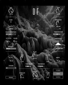
MIX: control the amount of direct signal and effected signal.
